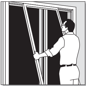
Insect screen removal from interior or exterior
