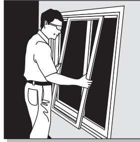
Removing the gliding sash
